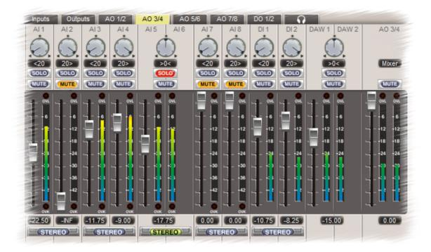
Each input channel has a fader, a high-resolution <u>peak meter</u>, with overload indication 0.05dB below clipping, plus mute and solo buttons and a pan-pot. By engaging the 'Stereo' button beneath an input pair, the pair is controlled by a single stereo fader, mute button and solo button, and the pan-pots are replaced by a single balance control. The DAW contribution and output strip are always in stereo mode.
