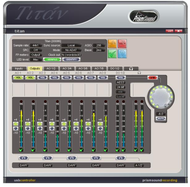
Whilst Titan can be controlled in a limited way from within the Mac or Windows operating system, or by some audio application programs, most of its detailed features can only be accessed using the Titan Control Panel app.
