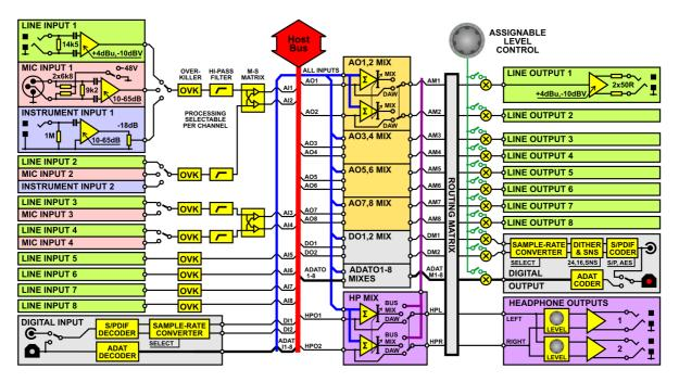
The figure above is a simplified block diagram of the Titan audio signal paths.
